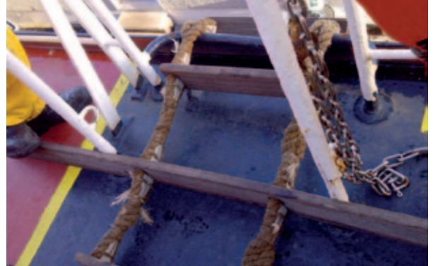
Poor and incorrect securing method
